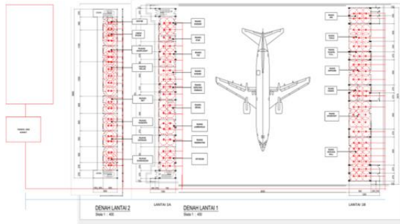
Figure 11: Sprinkler, Pump, and Water Tank Design
