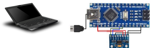
Gambar 11. Wiring Diagram Low-Cost Vibration Sensor
